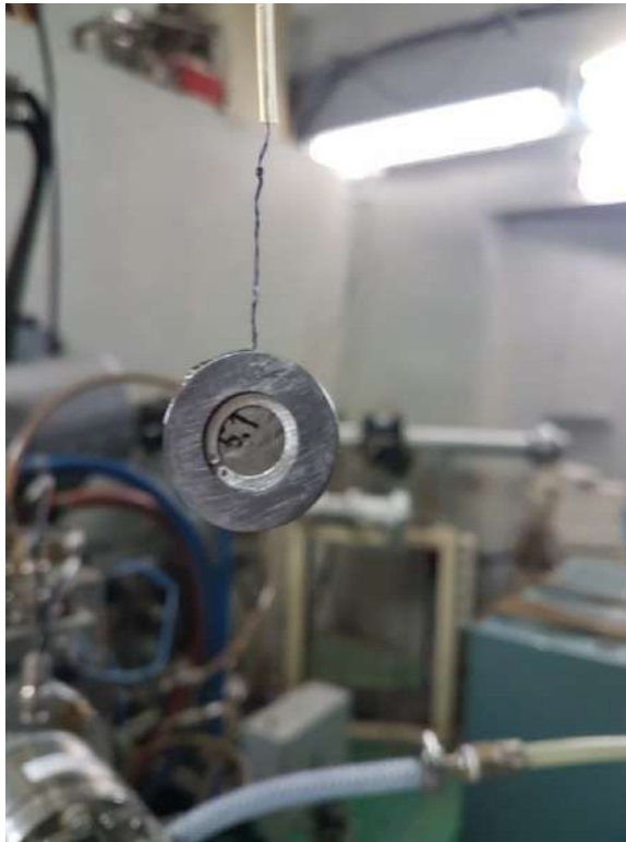
Figure 66 – Target holder: a tantalum substrate (400 \mu\text{m} thick) into which target foils are inserted, as well as foils for monitoring beam parameters. The foils are clamped by a special aluminum ring.
