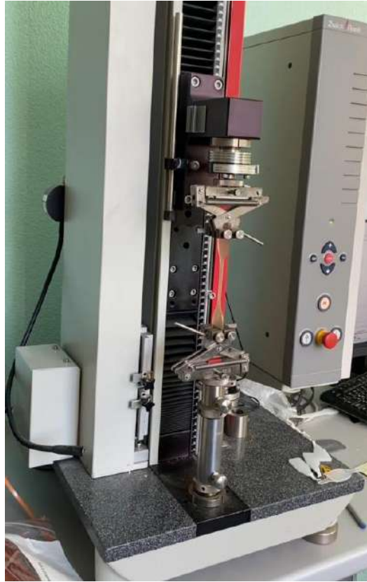
Figure 14 – Zwick/Roell Z5.0 tensile machine
