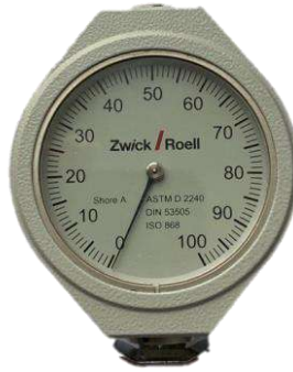
Figure 13 – Durometer for measuring polymer hardness on the shore a scale
