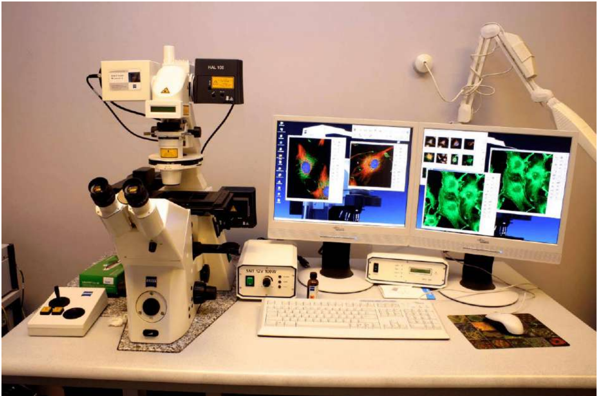
Figure 2. Laser immunofluorescence scanning confocal microscopy system
