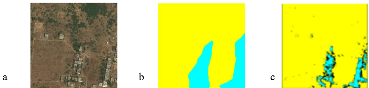
Figure 4.6. An example of segmentation of a satellite image: a) the original image; b) the marked mask; c) the result of segmentation. Color designations: yellow – agricultural land, blue — urban area, black — undefined area
