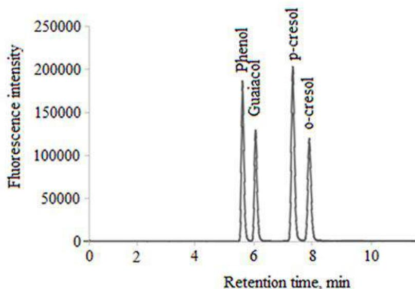
**Figure 13.** Chromatogram of solution of phenols ( $C_{\text{analyte}} = 1 \text{ mg/L}$ ).
