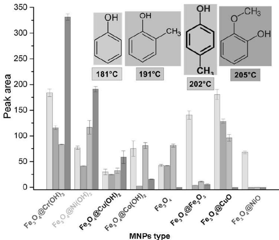
**Figure 25.** Effect of magnetic sorbent composition on the efficiency of headspace microextraction of phenol, *o*-cresol, *p*-cresol and guaiacol ( $C_{\text{analyte}} = 0.5 \text{ mg/kg}$ , sample weight – 0.5 g,  $n = 3$ ).
