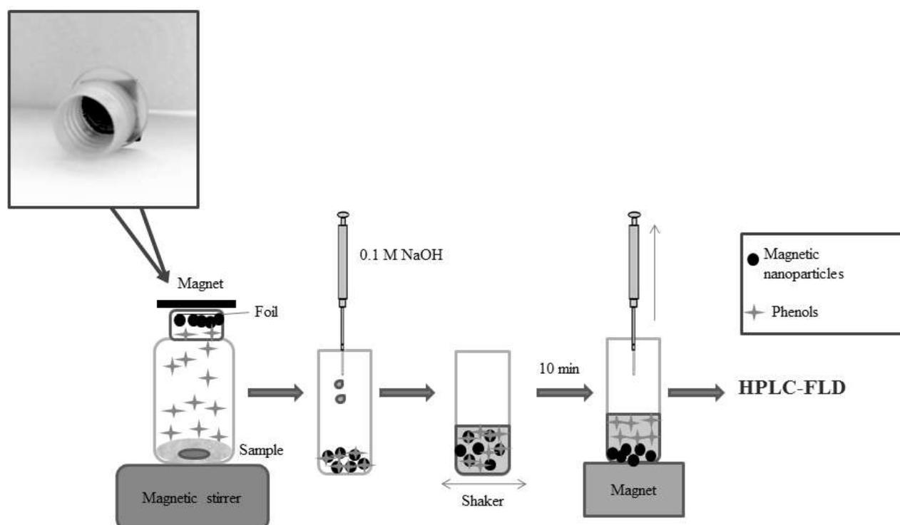
**Figure 23.** A combined method for the determination of volatile analytes, including static headspace microextraction on a magnetic sorbent, elution and subsequent chromatographic analysis.
