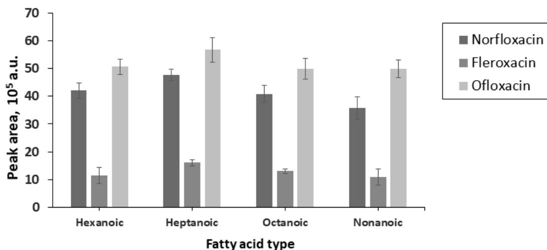
**Figure 34.** Effect of hydrogen bond donor in DES on chromatographic peak areas of fluoroquinolones ( $C_{\text{analyte}} = 200 \mu\text{g/L}$ , volume of extractant  $100 \mu\text{L}$ ,  $n = 3$ ).
