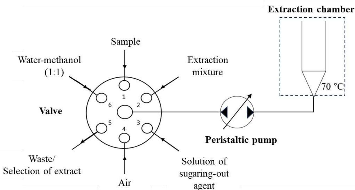
**Figure 49.** Automated DLLME based on phase transition of dispersive solvent for the analysis of water samples.
