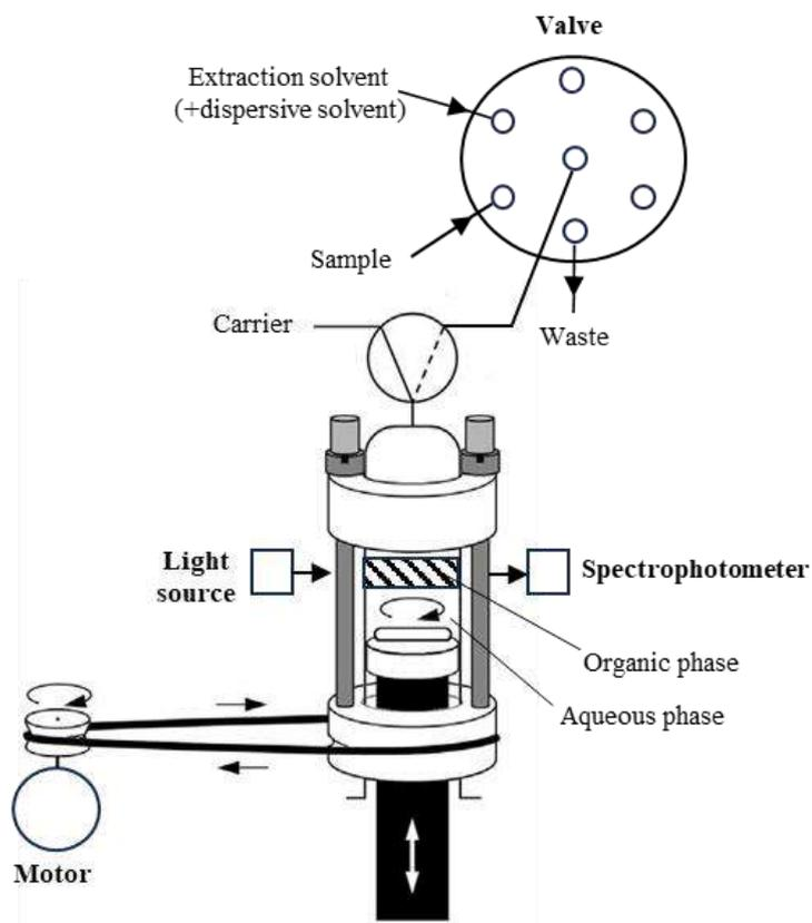
**Figure 9.** The scheme of lab-in-syringe with DLLME.
