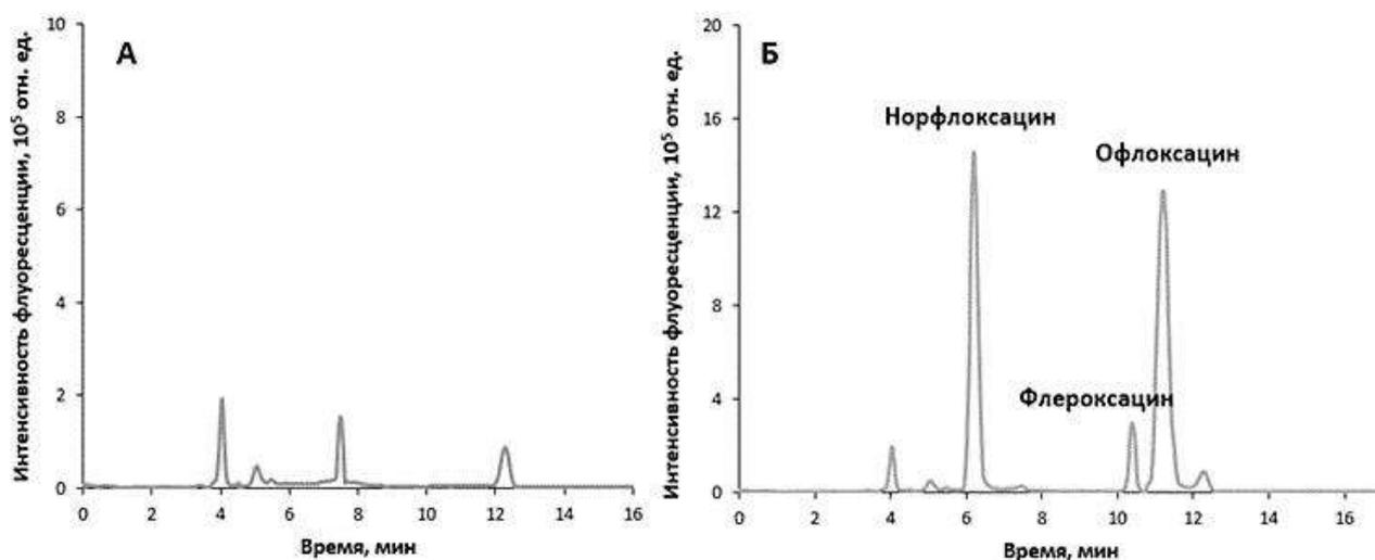
**Figure 12.** Chromatograms of the extracts of shrimp samples without additives (A) and spiked samples (B).
