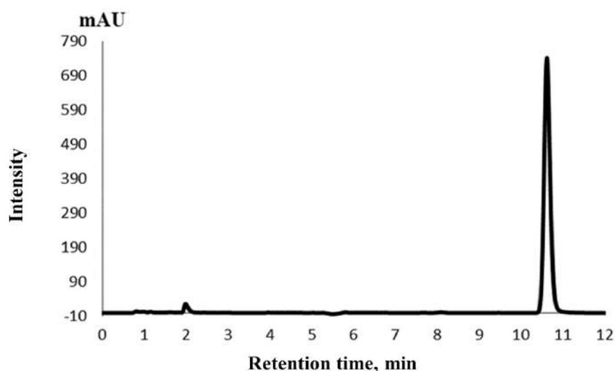
**Figure 44.** Chromatogram obtained during the determination of benzoic acid ( $C_{\text{analyte}} = 25 \text{ mg/L}$ ) in spiked juice sample using the developed method.
