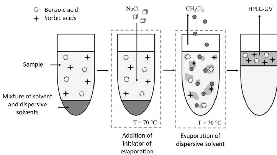
**Figure 46.** Scheme of DLLME with phase transition of dispersive solvent.
