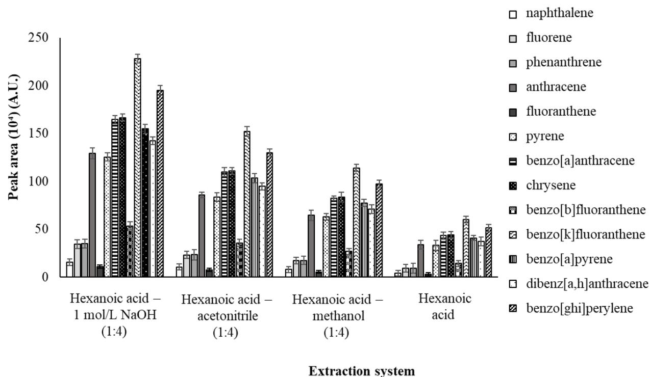
**Figure 59.** Comparison of the developed DLLME approach with the conventional DLLME and LLE ( $C_{\text{analyte}} = 5 \mu\text{g/L}$ ,  $n = 3$ ).
