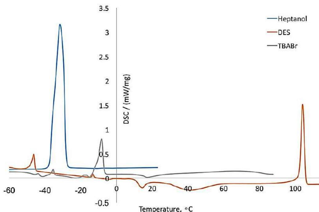
**Figure 32.** Differential scanning calorimetry record of DES (tetrabutylammonium bromide (TBABr) and heptanol at a 1:2 molar ratio) and its precursors.
