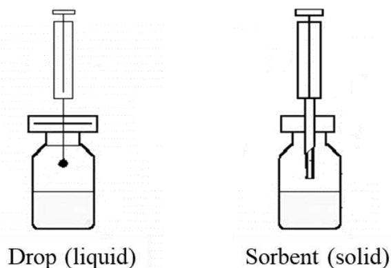
**Figure 6.** The scheme of headspace single-drop microextraction (left) and headspace solid phase microextraction (right).
