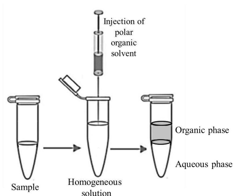
**Figure 3.** The scheme of HLME.
