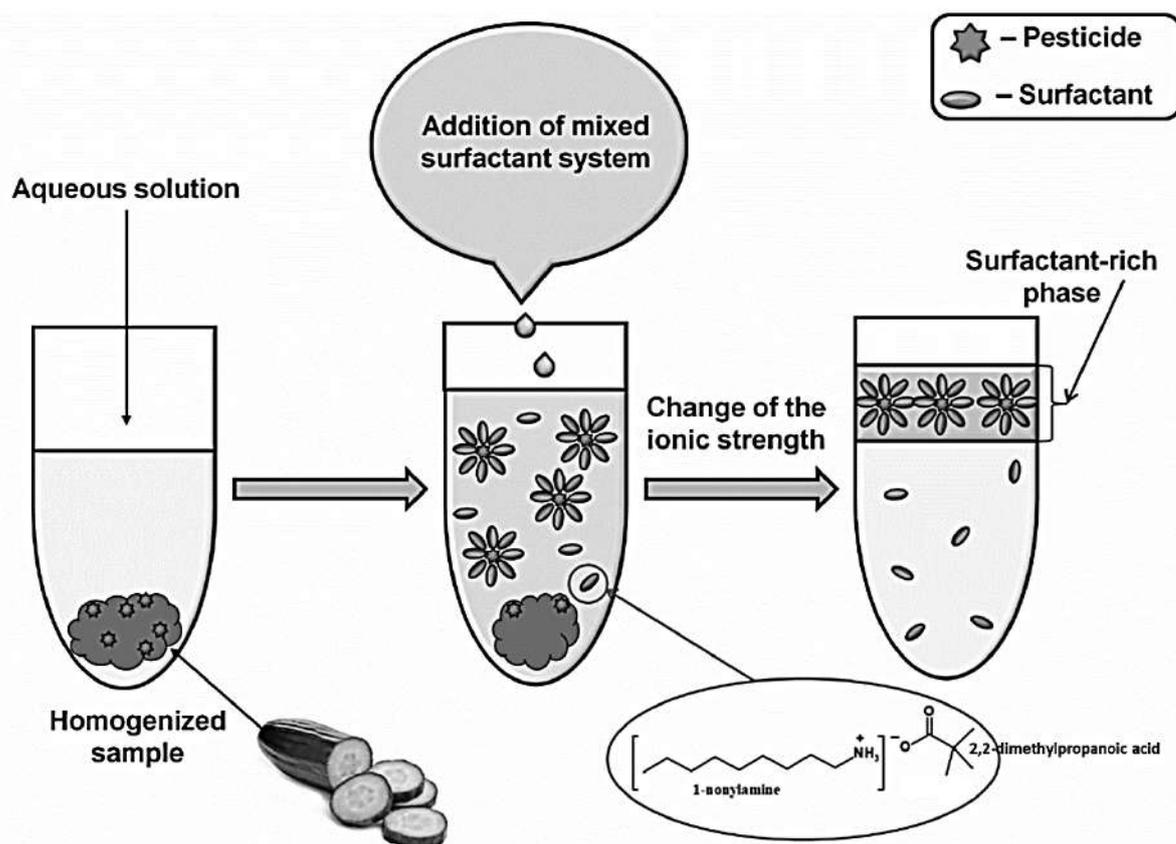
**Figure 42.** Micellar microextraction of pesticides from suspensions into a supramolecular solvent based on a primary amine and carboxylic acid.
