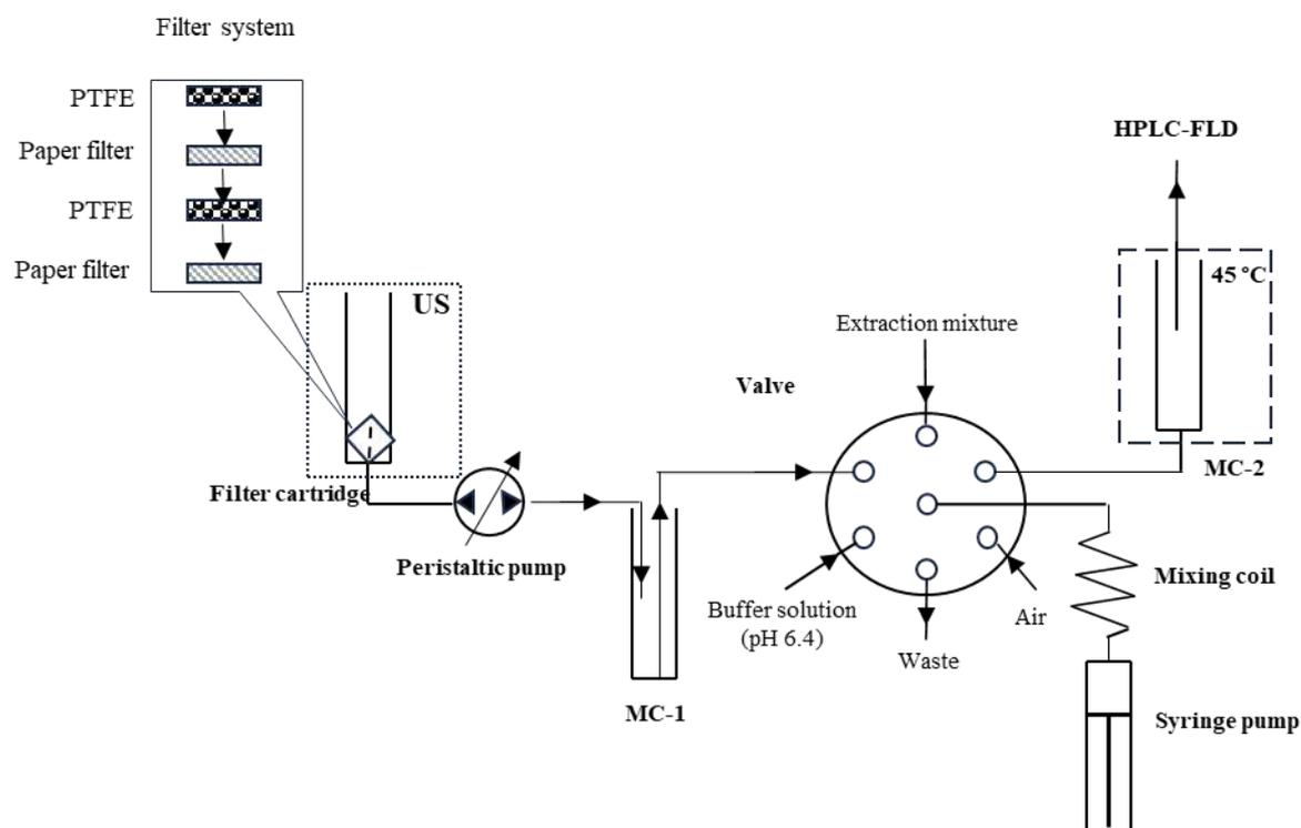
**Figure 51.** Automated sample preparation scheme including solid-liquid extraction of ofloxacin from a solid-phase sample, DLLME of the analyte from an aqueous solution, solvent exchange and subsequent HPLC-FLD analysis.
