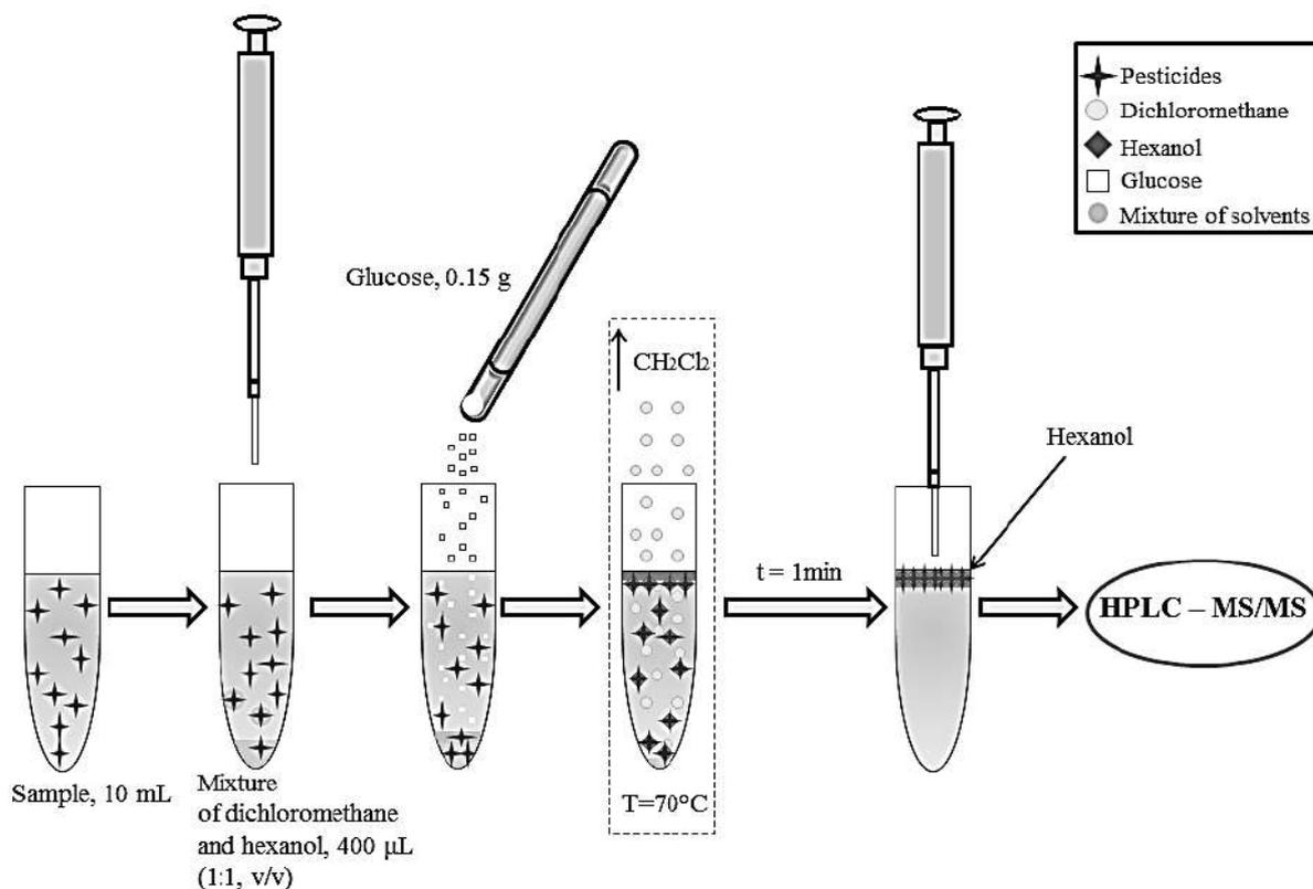
**Figure 48.** Scheme of the DLLME based on phase transition of volatile dispersive solvent for the determination of insecticides in wine.
