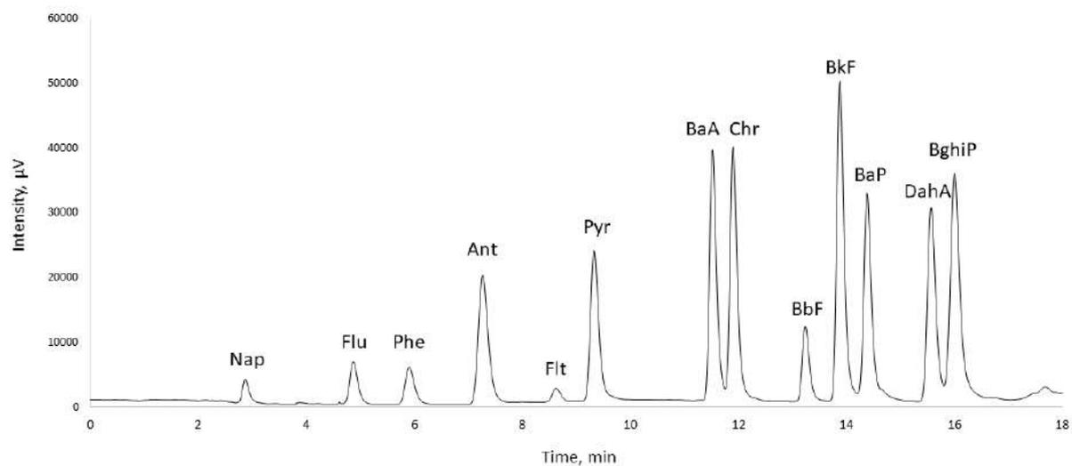
**Figure 17.** Chromatogram of an aqueous solution of a mixture of PAHs: BaA – benzo[a]anthracene, Chr – chrysene, BbF – benzo[b]fluoranthene, BaP – benzo[a]pyrene, BkF – benzo[k]fluoranthene, DahA – dibenz[a,h]anthracene, BghiP – benzo[ghi]perylene, Nap – naphthalene, Flu – fluorene, Phe – phenanthrene, Ant – anthracene, Flt – fluoranthene, Pyr – pyrene ( $C_{\text{analyte}} = 5 \mu\text{g/L}$ ).
