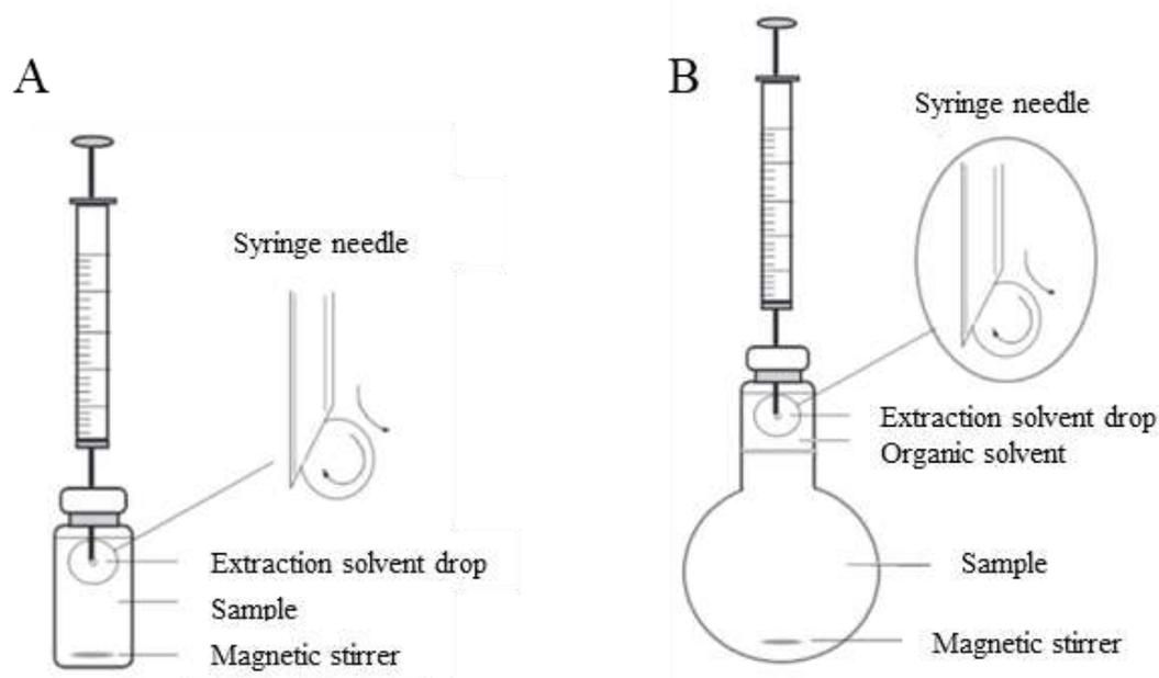
**Figure 2.** The scheme of two-phase (A) and three-phase (B) SDME.
