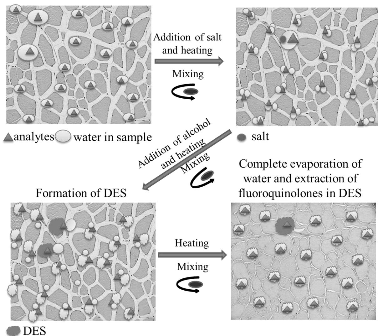
**Figure 30.** Mechanism of microextraction of fluoroquinolones from meat sample.
