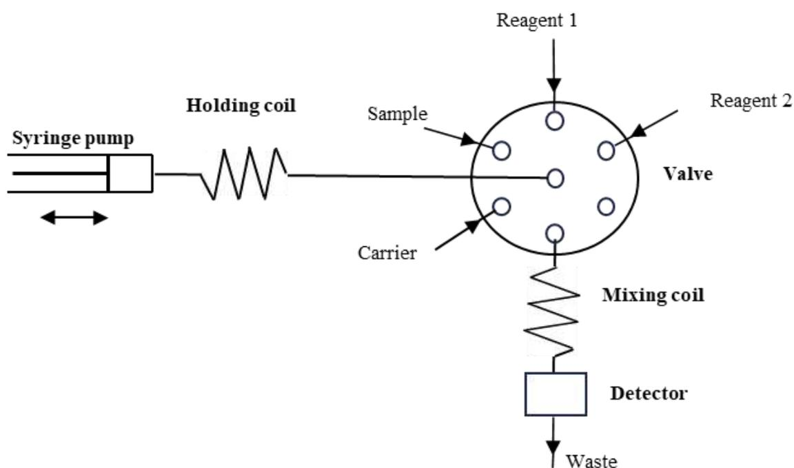
**Figure 8.** The scheme of SIA.
