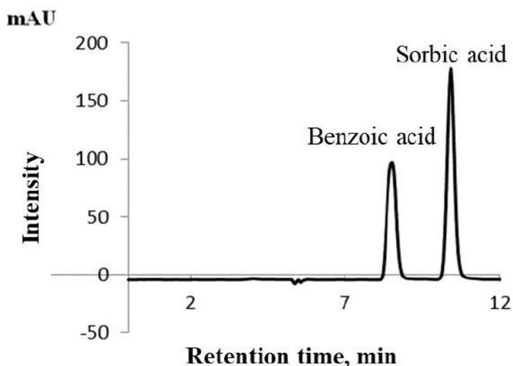
**Figure 15.** Chromatogram of the extract of a mixture of benzoic and sorbic acids ( $C_{\text{analyte}} = 25 \text{ mg/L}$ ).
