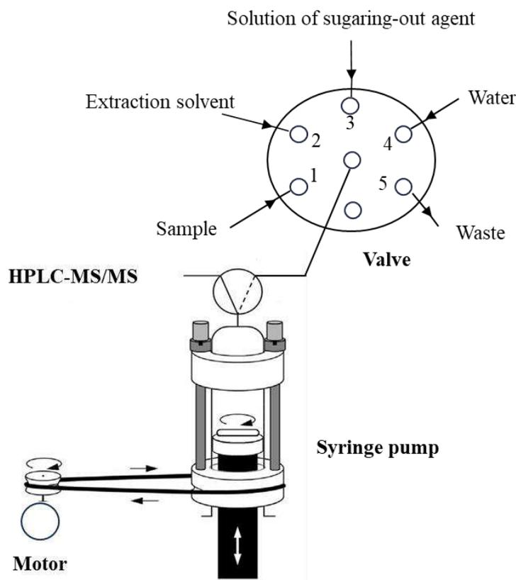
**Figure 54.** Scheme of in-syringe sugaring-out homogeneous liquid microextraction coupled with HPLC-MS/MS for the determination of pesticides.
