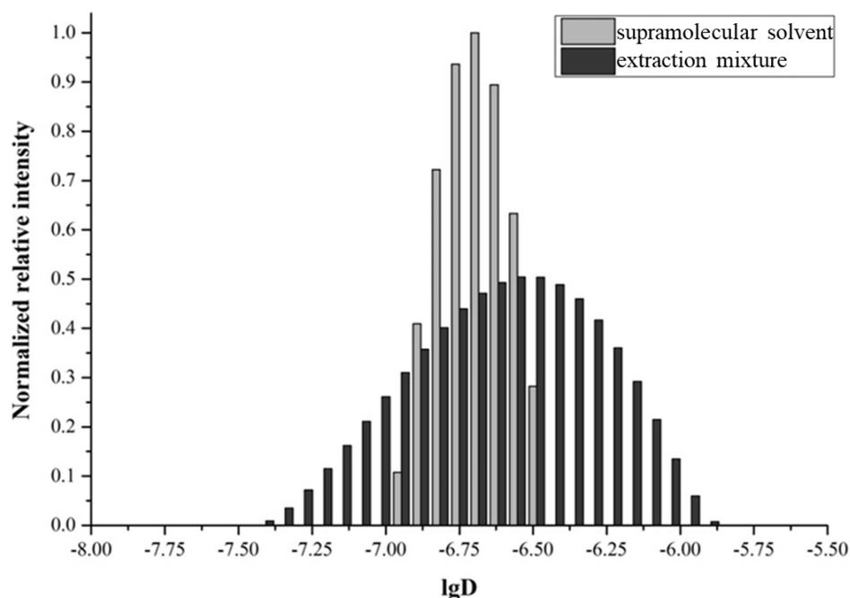
**Figure 41.** Distribution of the diffusion coefficients for supramolecular structures presented in the extraction mixture and the organic phase ( $T = 293 \text{ K}$ , a scattering angle of  $90^\circ$ ).
