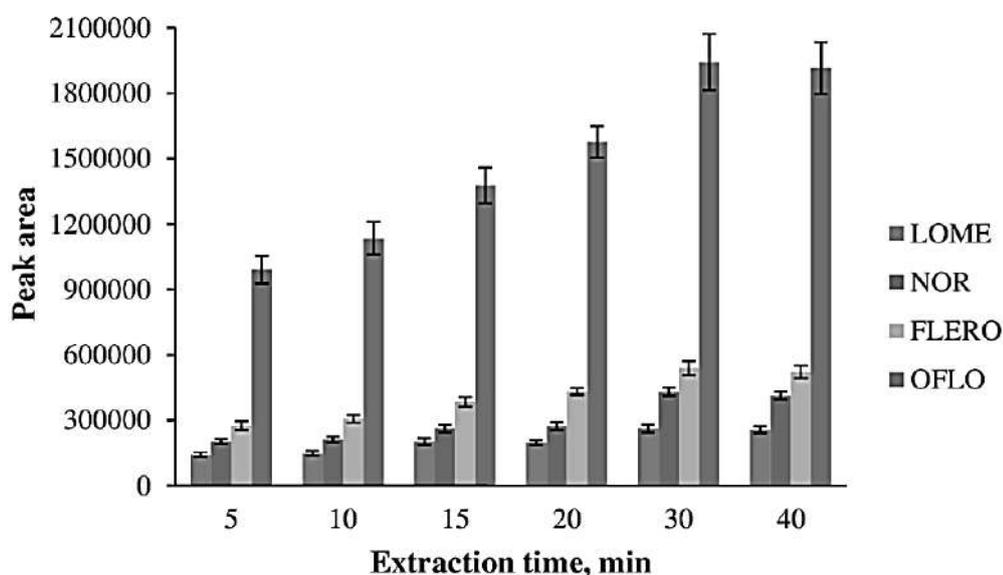
**Figure 29.** Effect of extraction time on the chromatographic peak areas of fluoroquinolones ( $C_{\text{analyte}} = 100 \mu\text{g/L}$ ;  $n = 3$ ).
