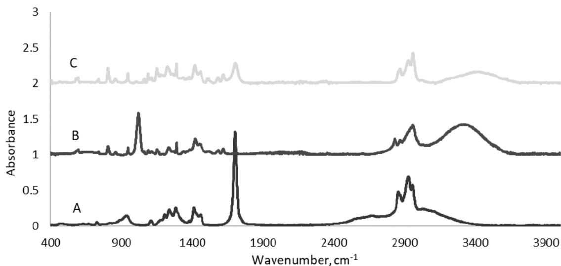
**Figure 37.** FT-IR spectra of heptanoic acid (A), thymol (B) (dissolved in methanol 1:1) and the obtained DES phase (C) after the DLLME.
