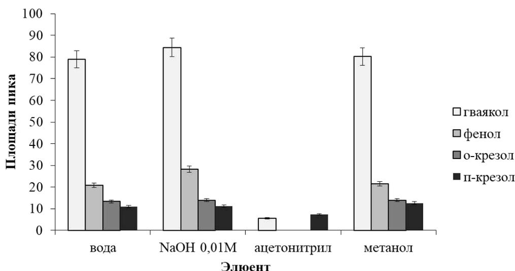
**Figure 26.** Efficiency of the elution process of phenols from magnetic nanoparticles  $\text{Fe}_3\text{O}_4@\text{Cr}(\text{OH})_3$  using different eluents ( $C_{\text{analyte}} = 0.1 \text{ mg/kg}$ ,  $n = 3$ ).
