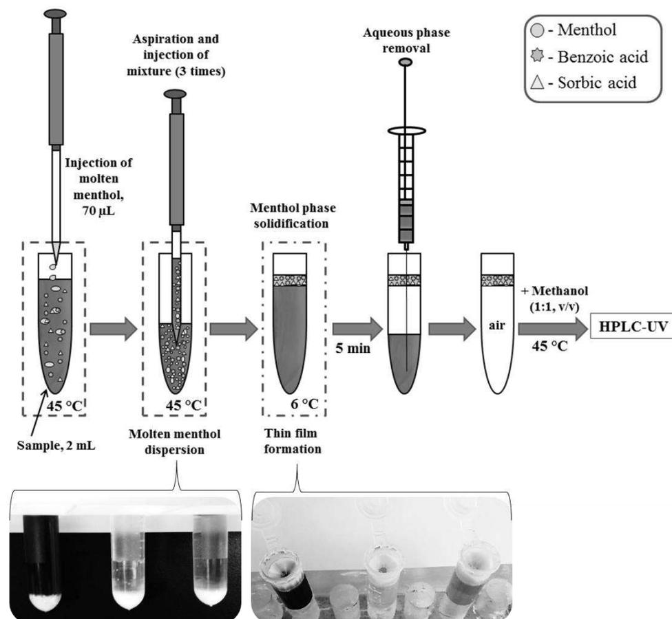
**Figure 45.** DLLME based on the phase transition of the extraction solvent (liquid – solid).
