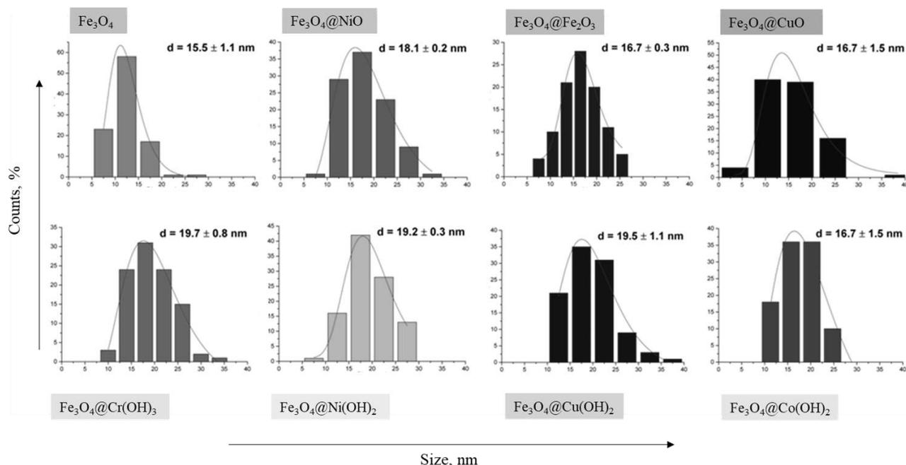
**Figure 24.** Size distribution of synthesized magnetic NPs.
