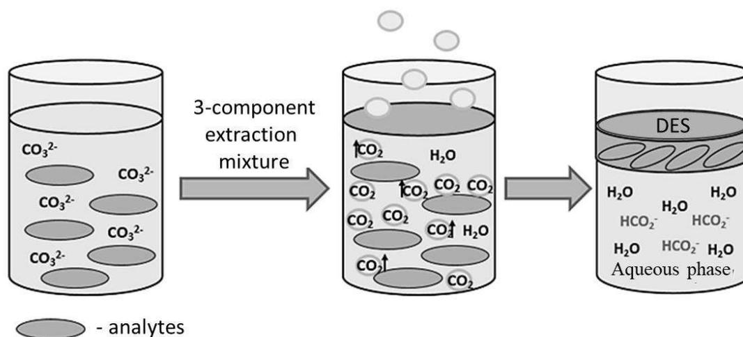
**Figure 33.** Dispersive liquid-liquid microextraction into a deep eutectic solvent with dispersion of the gas phase formed *in situ*.
