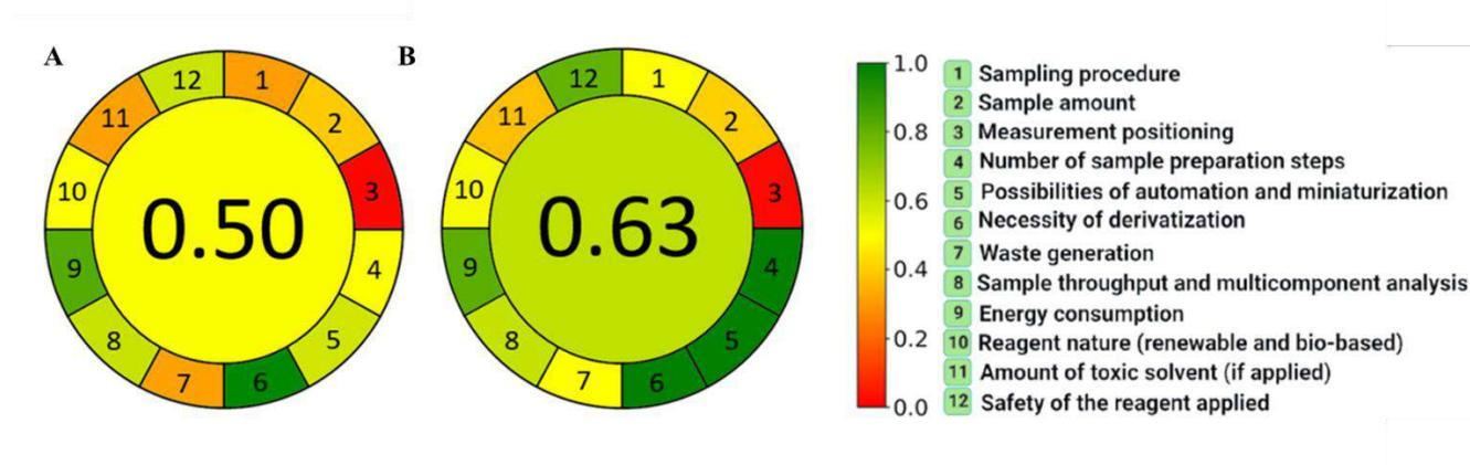
**Figure 52.** Indexes of greenness assessment for manual (A) and automated (B) approaches of DLLME with phase mixing by carbon dioxide formed *in situ*.
