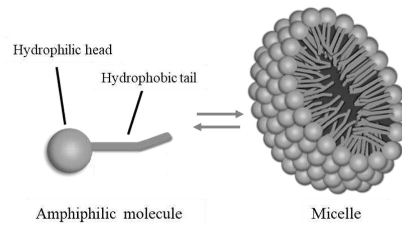
**Figure 4.** Schematic representation of an amphiphilic surfactant molecule and micelle formation from monomers.
