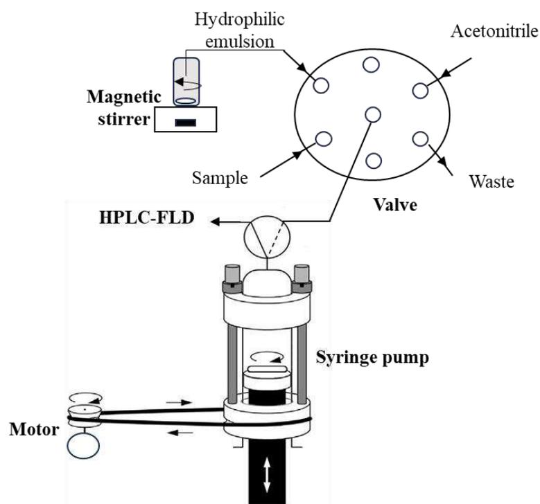
**Figure 58.** Automated scheme of the DLLME using salt of medium-chain fatty acid as dispersive anionic surfactant.
