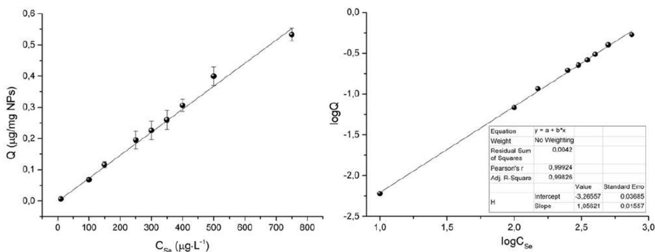
**Figure 22.** H<sub>2</sub>Se adsorption isotherm for bare Fe<sub>3</sub>O<sub>4</sub> nanoparticles (left) (5 mg of MNPs) and Freundlich model linearization (right).
