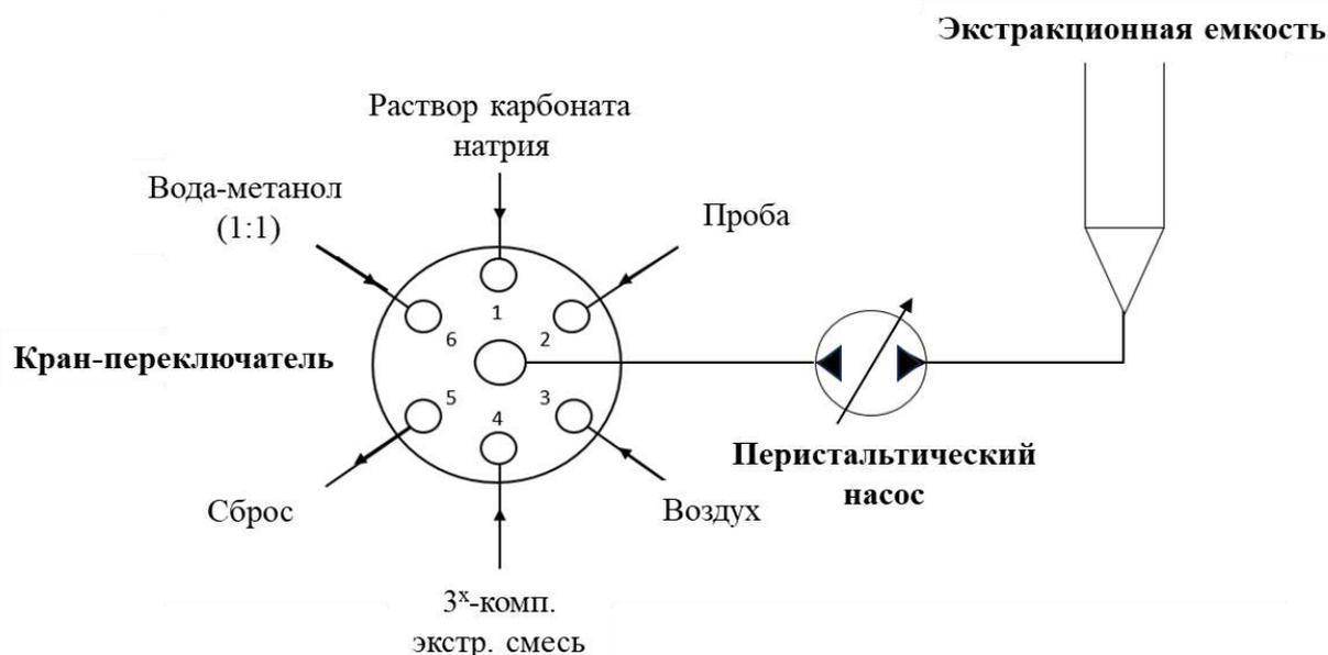
**Figure 51.** Scheme of automated DLLME in DES with phase mixing by carbon dioxide formed *in situ* for the analysis of water samples.
