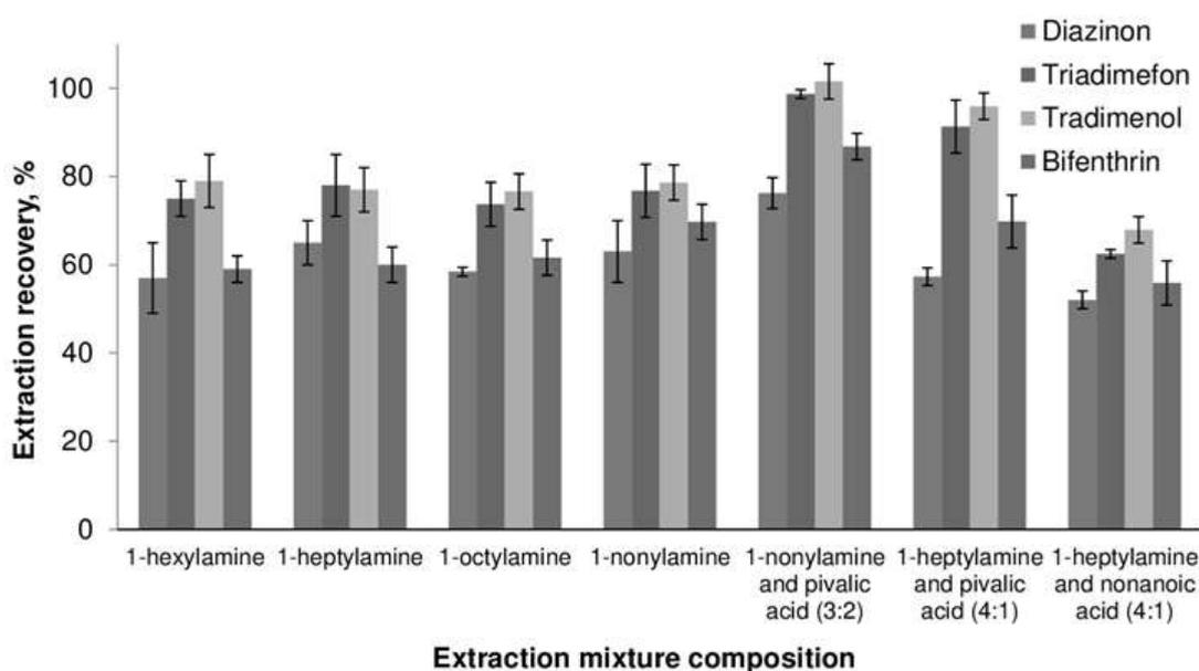
**Figure 39.** Effect of extraction mixture composition on the degree of pesticide extraction, *pivalic acid* = 2,2-dimethylpropanoic acid ( $C_{\text{analyte}} = 100 \mu\text{g/L}$ ,  $n = 3$ ).
