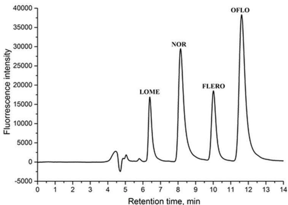
**Figure 14.** Chromatogram of the extract of a mixture of fluoroquinolones: lomefloxacin (LOME), norfloxacin (NOR), fleroxacin (FLERO) and ofloxacin (OFLO) ( $C_{\text{analyte}} = 100 \mu\text{g/L}$ ).
