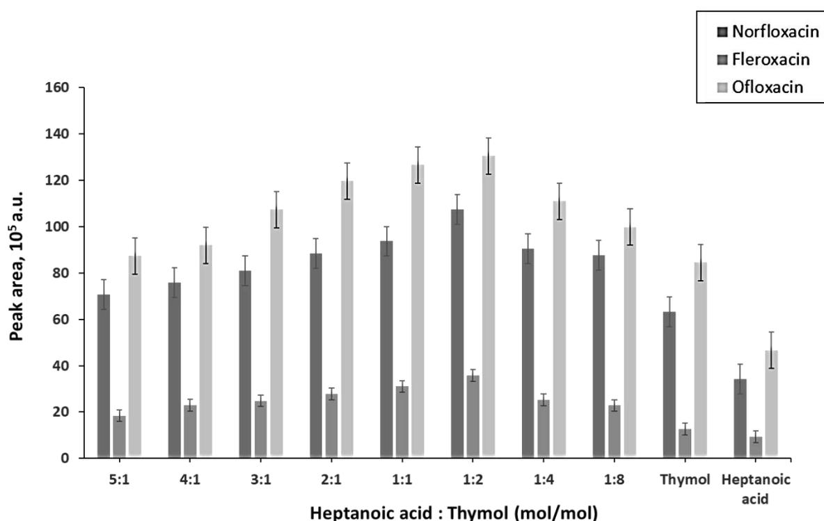
**Figure 36.** The influence of the ratio of DES precursors (heptanoic acid and thymol), as well as the individual precursors, on the areas of chromatographic peaks of fluoroquinolones ( $C_{\text{analyte}} = 200 \mu\text{g/L}$ , volume of extractant  $100 \mu\text{L}$ ,  $n = 3$ ).
