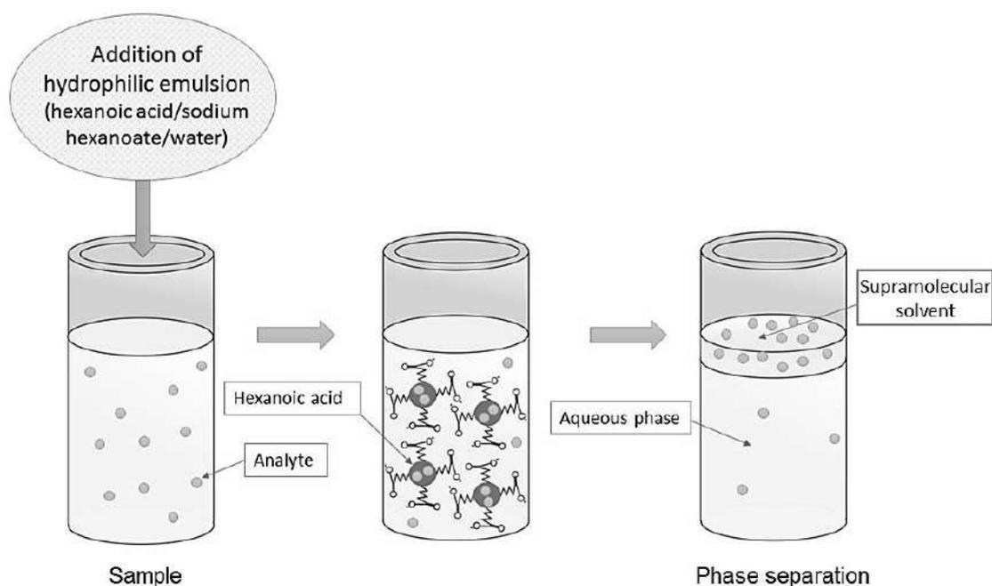
**Figure 56.** Scheme of DLLME using salt of medium-chain fatty acid as dispersive anionic surfactant.
