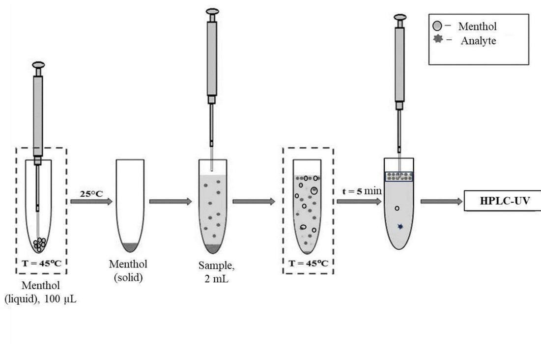
**Figure 43.** DLLME based on the phase transition of the extraction solvent (solid – liquid).
