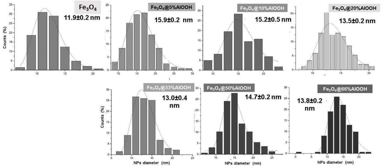
**Figure 20.** Size distribution of synthesized magnetic NPs.
