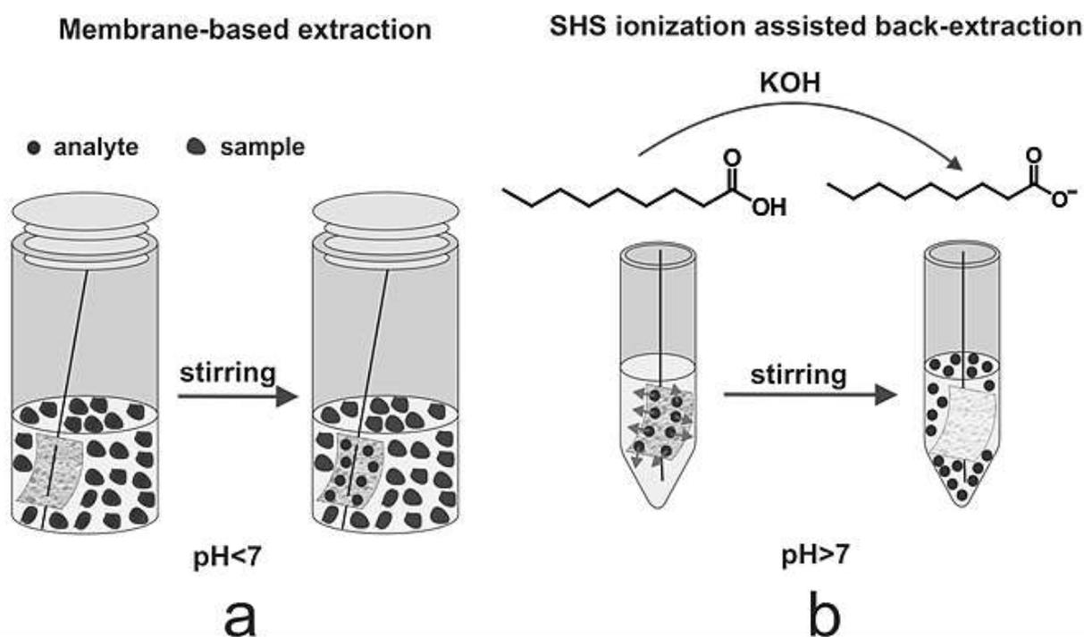
**Figure 27.** Scheme of microextraction of fluoroquinolones from suspended samples on membranes impregnated with medium-chain fatty acid: extraction (a) and back-extraction (b) processes.
