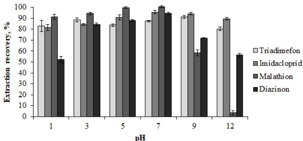
**Figure 55.** Effect of pH on the extraction recovery of target analytes ( $C_{\text{diazinon}} = 1 \mu\text{g/L}$ ,  $C_{\text{malathion}} = 10 \mu\text{g/L}$ ,  $C_{\text{triadimefon}} = 10 \mu\text{g/L}$ ,  $C_{\text{imidacloprid}} = 50 \mu\text{g/L}$ ,  $21 \text{ }^\circ\text{C}$ ,  $n = 3$ ).
