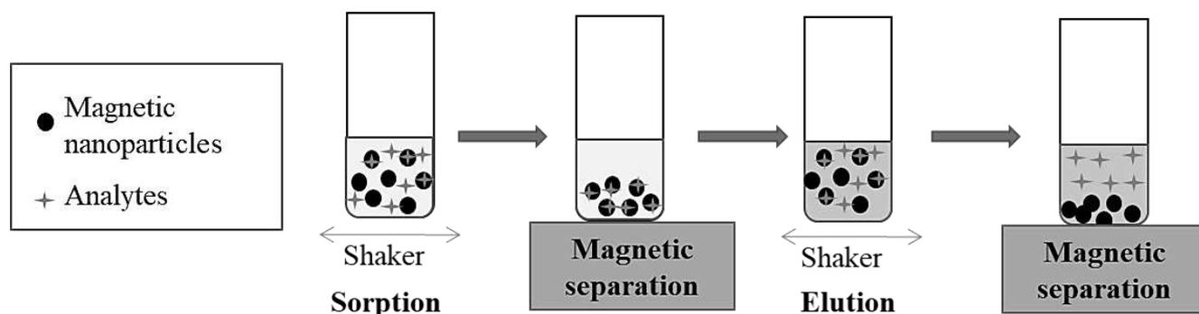
**Figure 5.** Solid-phase microextraction on magnetic nanoparticles.
