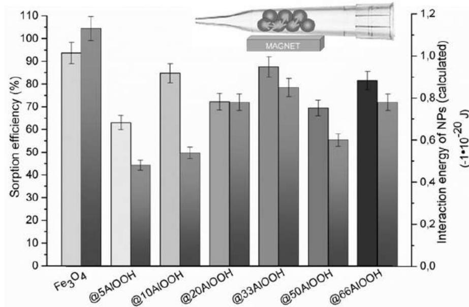
**Figure 21.** Sorption efficiency (left) and interaction energy values (right) in gas phase under the external magnetic field for MNPs synthesized (5 mg of MNPs) ( $n = 3$ ).
