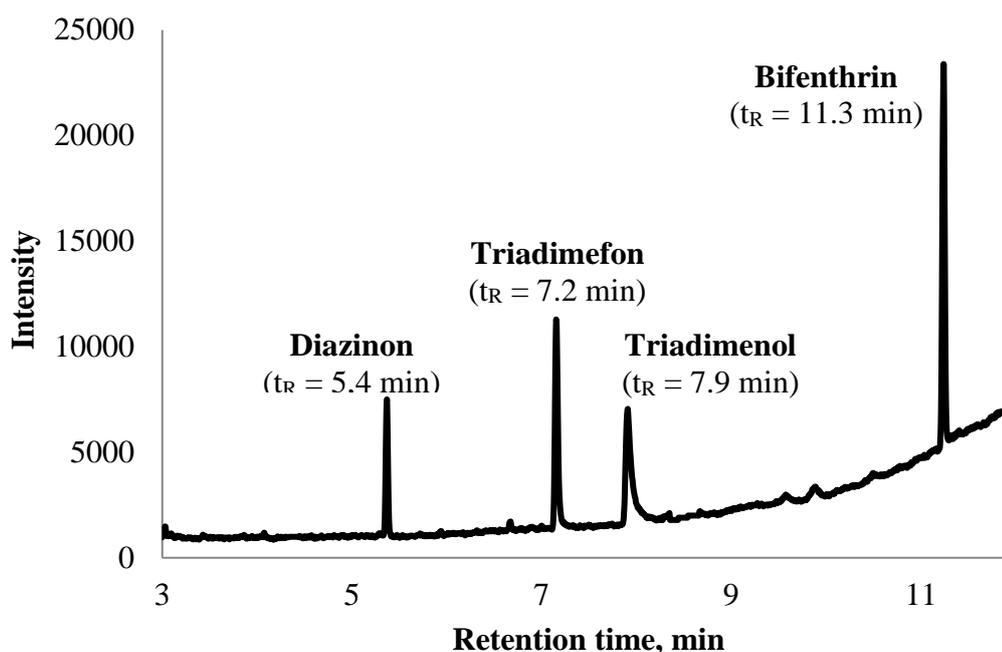
**Figure 16.** Chromatogram of a standard solution of a mixture of pesticides ( $C_{\text{analyte}} = 100 \mu\text{g/L}$ ).
