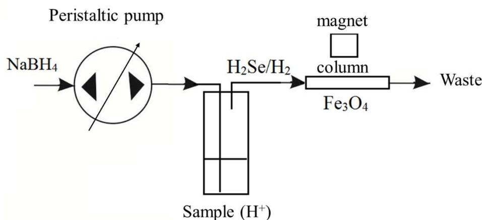
**Figure 19.** Scheme of dynamic headspace microextraction of volatile analyte on magnetic nanoparticles.
