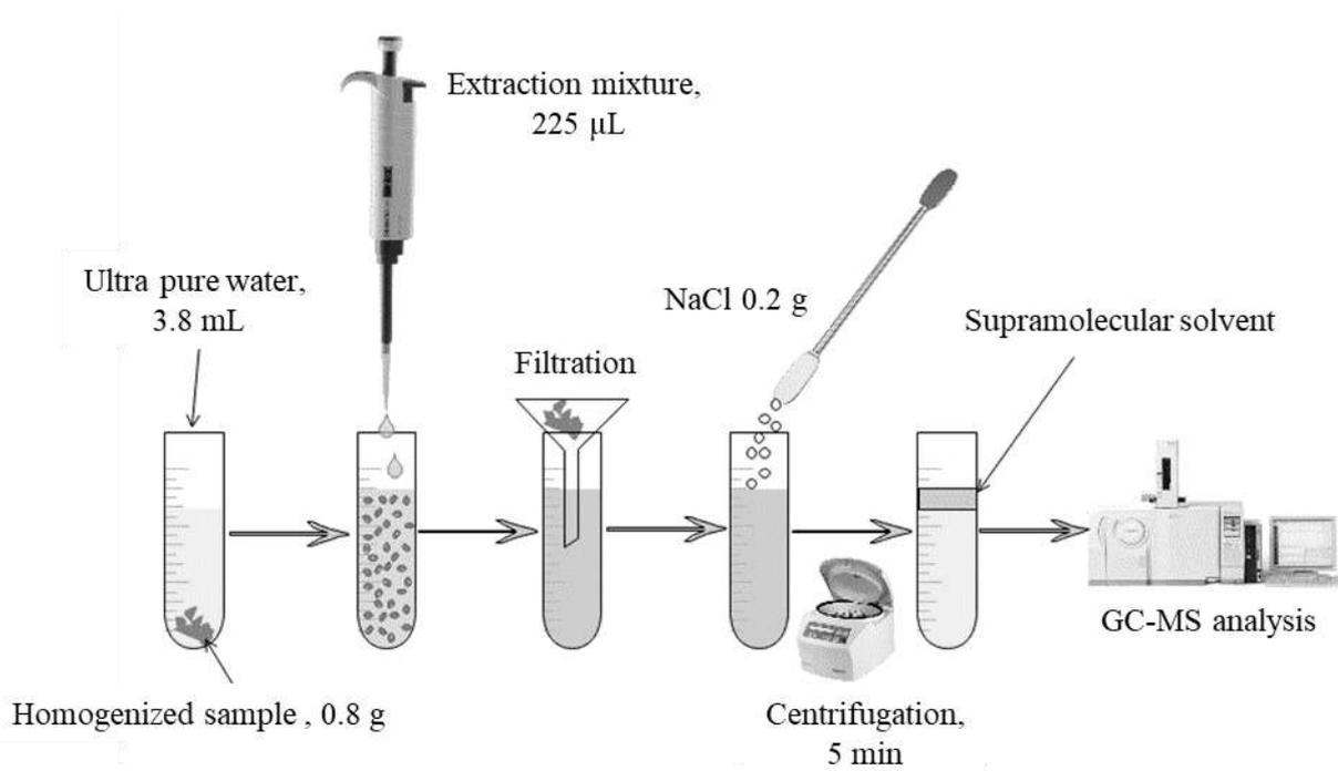
**Figure 40.** A combined scheme for the analysis of solid-phase food samples, including micellar microextraction and subsequent GC-MS analysis.
