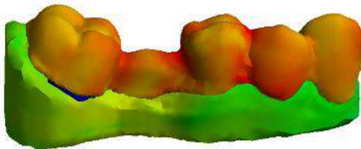
Figure 118 - Elastic shear deformation with beam reinforcement
