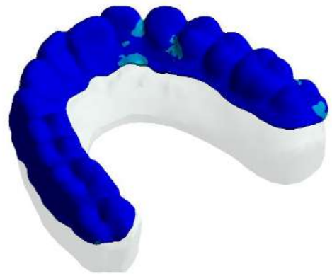
Figure 124 - Elastic aligner deformation with straight Cut
