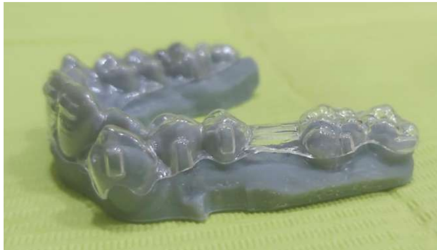
Figure 151 - Irreversible deformation of aligner with standard design
