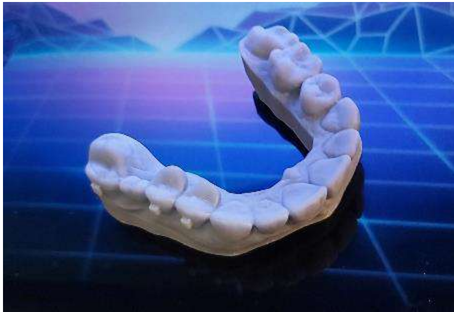
Figure 138 - Printed 3D model on the Anycubic Photon S 3D SLA printer after processing in isopropanol and UV cure
