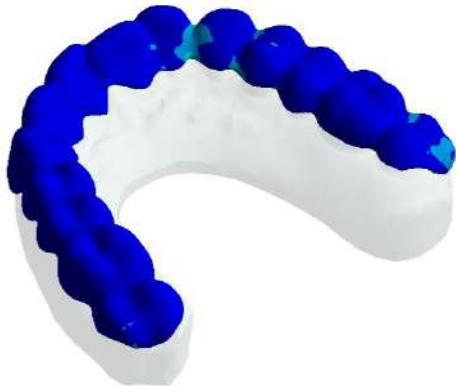
Figure 123 - Elastic aligner deformation with scalloped margin
