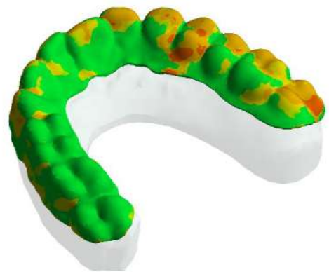
Figure 126 - Straight cut aligner shear Stress
