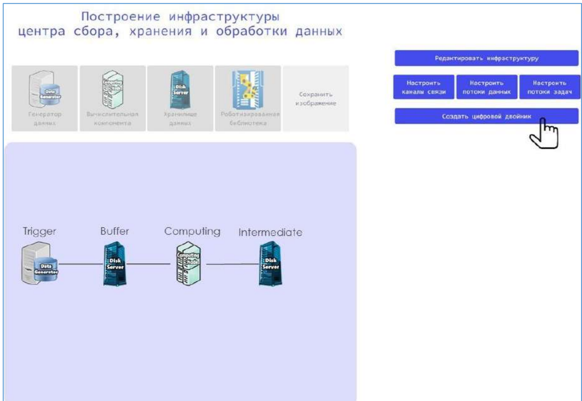
Figure 73. Computational system for online data filtering of SPD experiment
