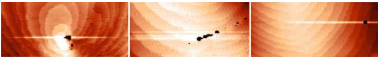
Figure 2.25 – Artefacts caused by the tip falling into dislocation channels of considerable width
