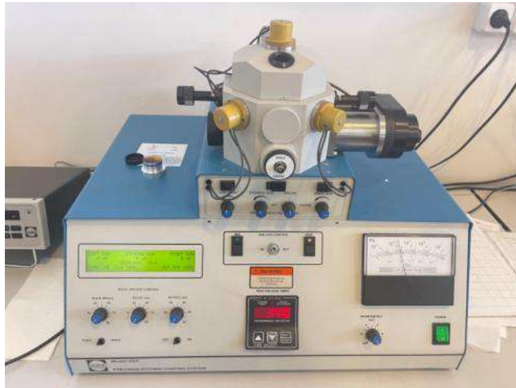
Figure 27. Universal system for sample preparation "GatanPECSModel 682" (Precision etching coating system)
