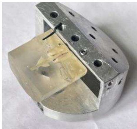
Figure 28. The process of fixing the sample with a carbon tape to a standard metal puck (a) and placing it on the microscope slide (b)
