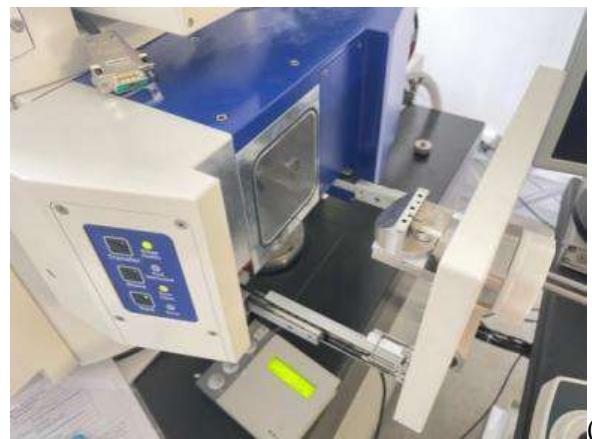
Figure 28. The process of fixing the sample with a carbon tape to a standard metal puck (a) and placing it on the microscope slide (b)
