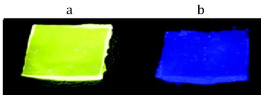
Figure 5 – Optical photographs of thermo-photoluminescent silicone rubbers at 80 ( a ) and 120°C ( b ) [78]
