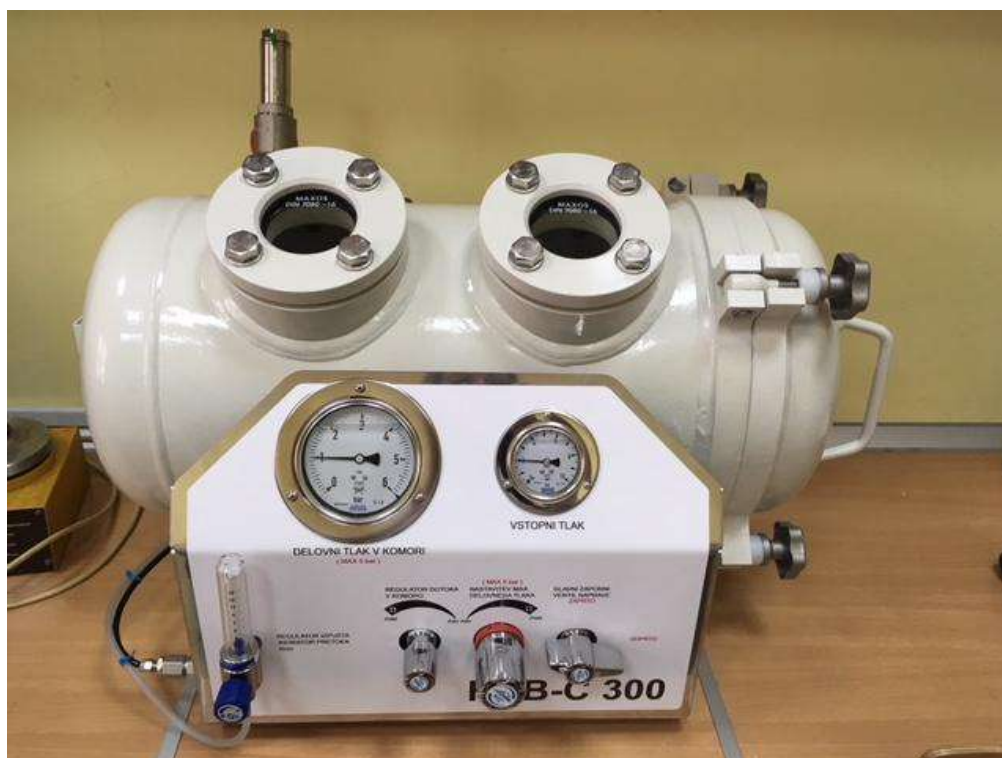
Figure 2 - Special oxygenation chamber for small experimental animals.
