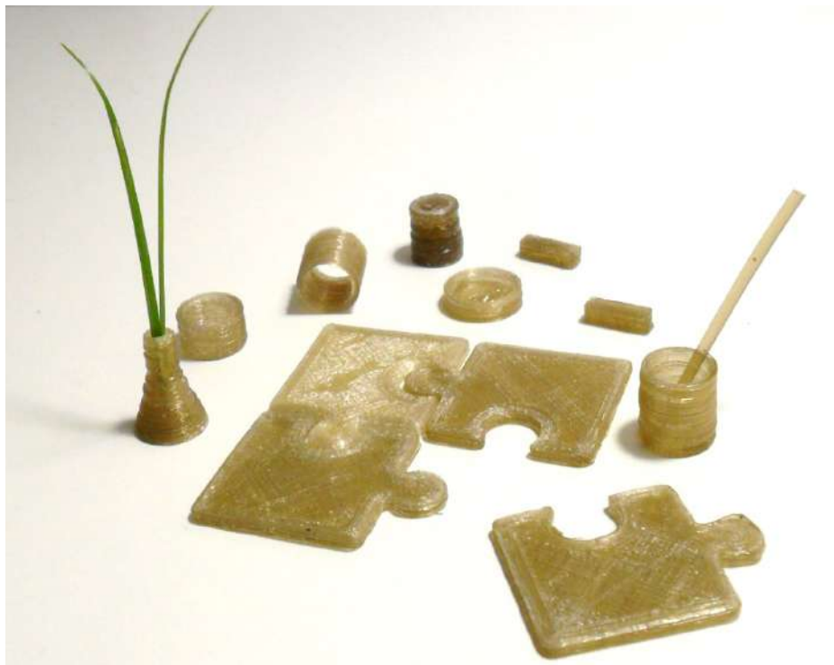
Figure 2.16. Objects printed on a 3D printer from PMVE+M1-30 material
