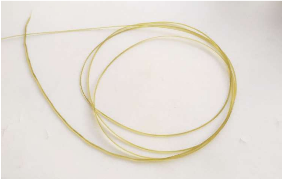
Figure 2.15. Filament from PMVE+M1-30 material
