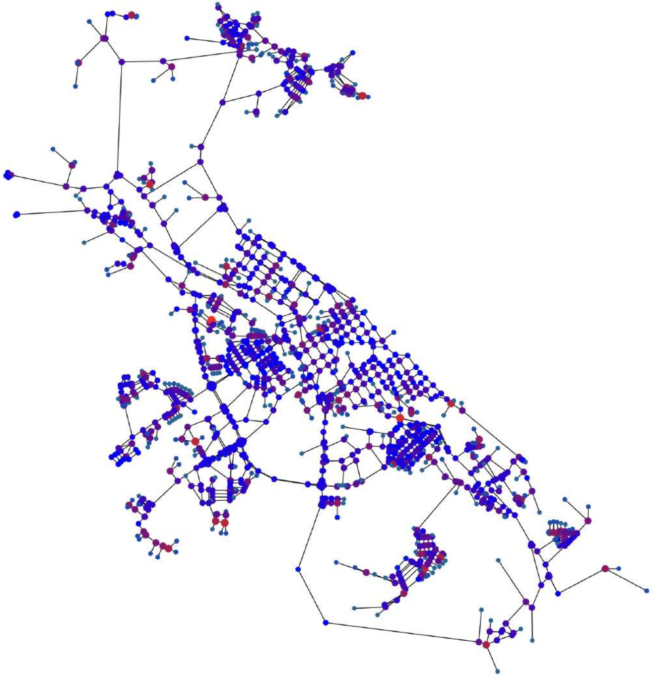
Figure 3.13 — Heatmap of vertex ranks of unweighted transport graph, PageRank method
