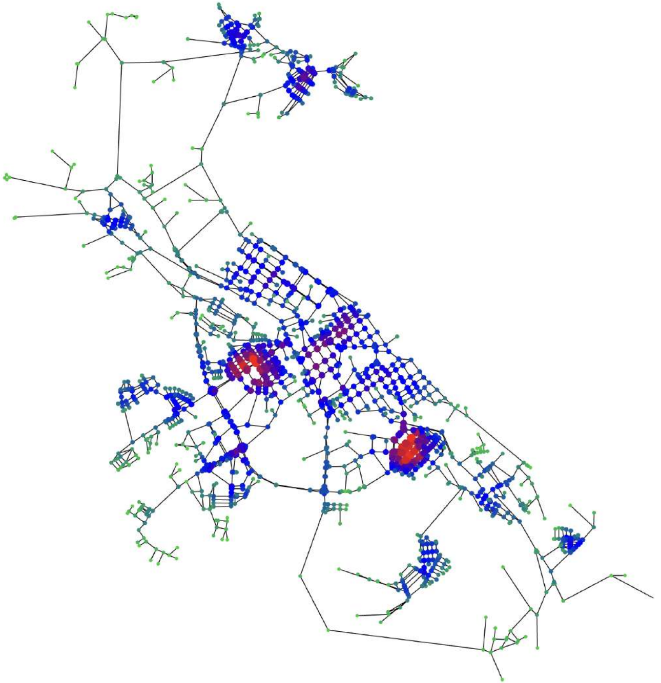
Figure 3.12 — Heat map of transport graph vertex ranks based on absolute potential values (weighted edges)
