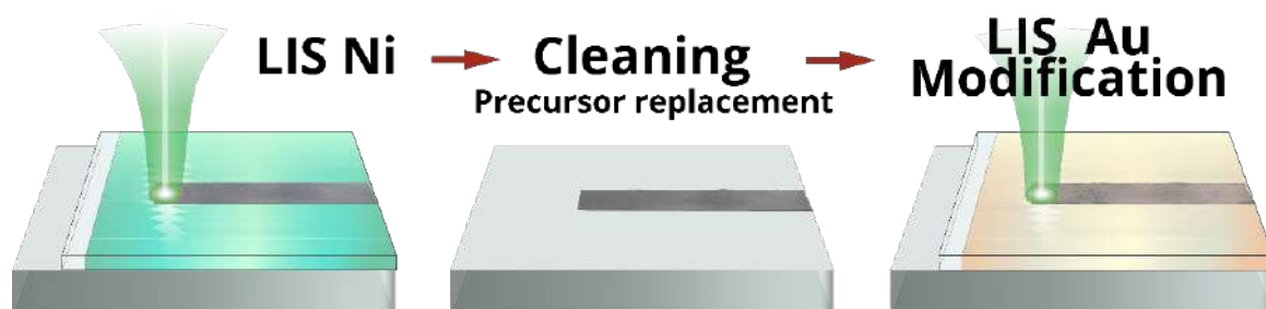
Figure 19 - Laser-induced synthesis at the interface between substrate and liquid reaction medium
