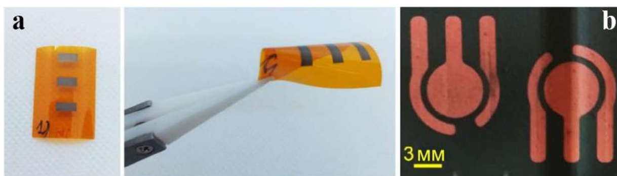
Figure 65 - Photographs of (a) Ni-NiO and (b) Cu-Cu x O y electrodes fabricated on the surface of polyimide (black background corresponds to the area not exposed to laser irradiation prior to the unirradiated ink removal procedure).
