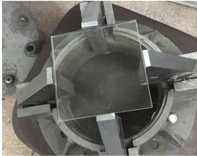
Fig. 5.1. The sample mounting device: four grips fixing the specimen.
