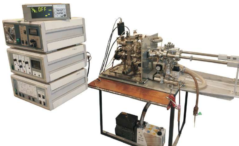
Figure. 3.2. – Magnetic-sector mass-spectrometric complex MSU-G-01-M (IPGG RAS)
