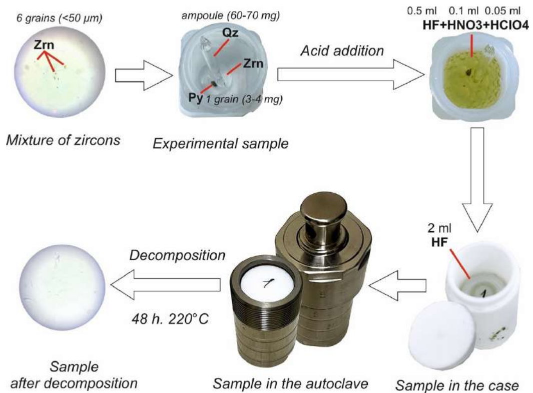
Figure 6.4. – Experiment on the decomposition of a pyrite sample (pyrite, quartz ampoule, zircon mixture), including difficult to dissolve uranium–bearing minerals, under pressure in autoclaves.
