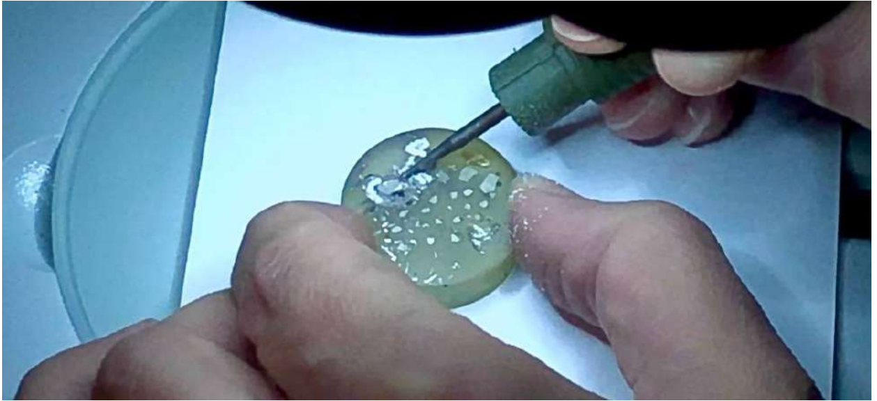
Figure 6.4. – Local sampling of pyrite from an ashlip with a diamond miniborer
