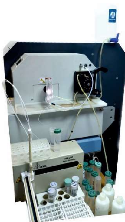
Figure. 3.3. – ELEMENT XR magnetic–sector inductively coupled plasma mass spectrometer (GEOCHI RAS)
