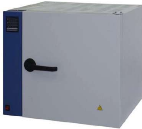
Figure 12 LOIP LF-60/350-VS2 laboratory drying oven used in the thermal cycling test
