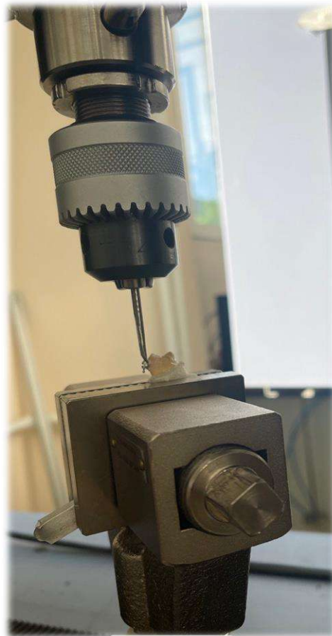
Figure 9 Extracted tooth with bonded bracket placed in an acrylic block mounted in the clamps of the testing machine
