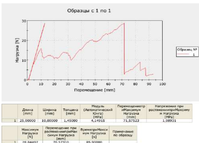
Figure 3.2.1.5.4 – Indicators of breaking load and stretching of the prosthesis-tissue complex for Ventralight ST endoprosthesis samples. a – animal 1 (sample 1 along the loop column); b – animal 2 (sample 1 along the loop row, samples 2 and 3 along the loop column); c – animal 3, endoprosthesis 1 (sample 1 along the loop column); d – animal 3, endoprosthesis 2 (sample 1 along the loop row, sample 2 along the looped column).
