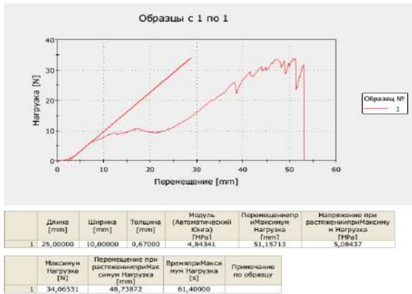
Figure 3.2.1.5.4 – Indicators of breaking load and stretching of the prosthesis-tissue complex for Ventralight ST endoprosthesis samples. a – animal 1 (sample 1 along the loop column); b – animal 2 (sample 1 along the loop row, samples 2 and 3 along the loop column); c – animal 3, endoprosthesis 1 (sample 1 along the loop column); d – animal 3, endoprosthesis 2 (sample 1 along the loop row, sample 2 along the looped column).
