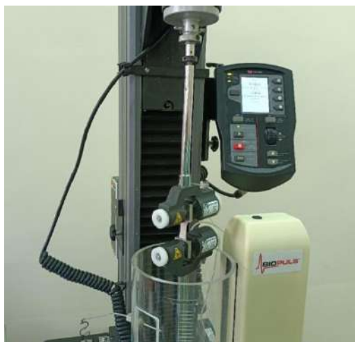
Figure 2.1.1.1 – Conducting physical and mechanical tests of the sample using the Instron 5900 testing machine.
