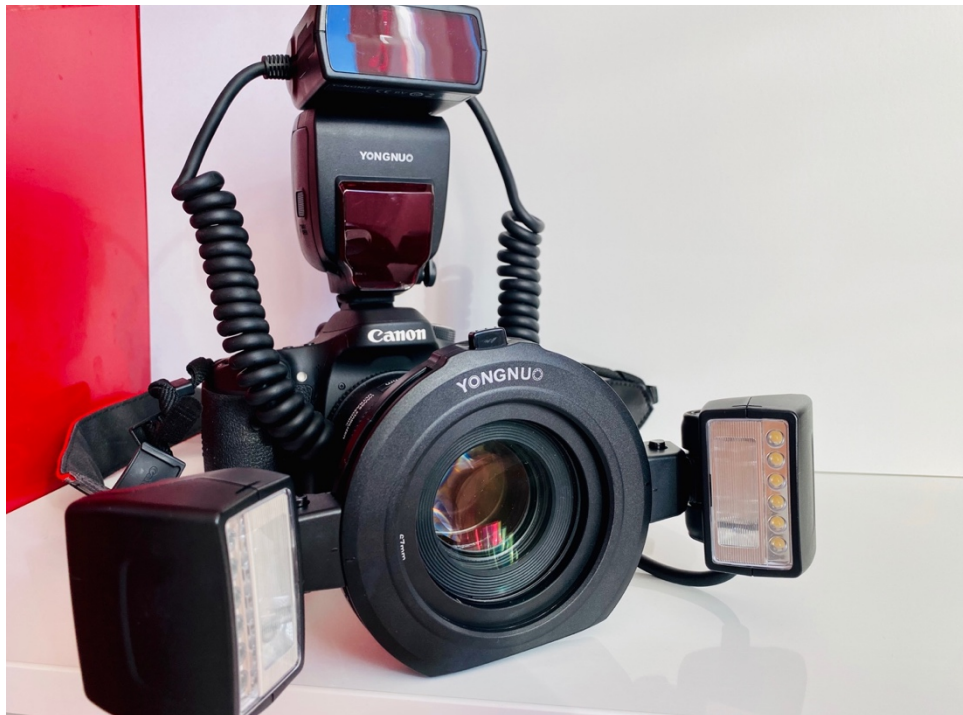
Figure 8. Canon80D camera with a macro lens for dental photos and bipolar flash lamp
