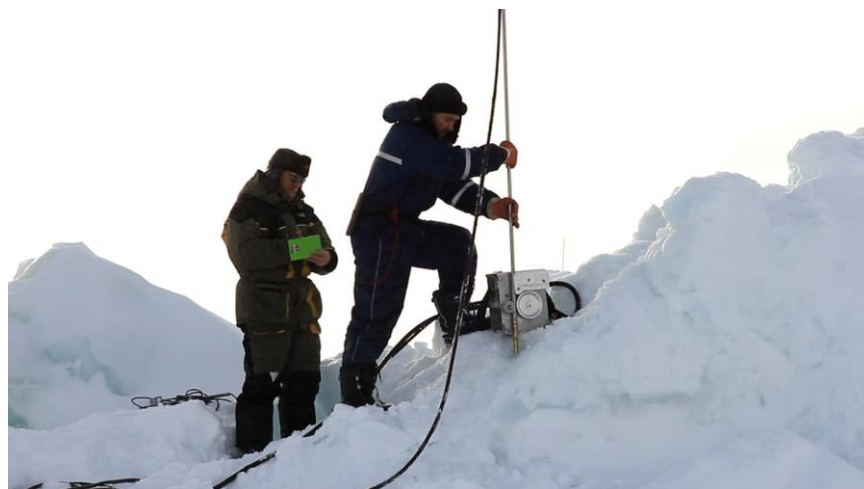
Figure 1.8 – Drilling team on the slope of the ice ridge sail. The drilling operator puts the thermal drill close to the measuring wheel of the transducer on the measuring box
