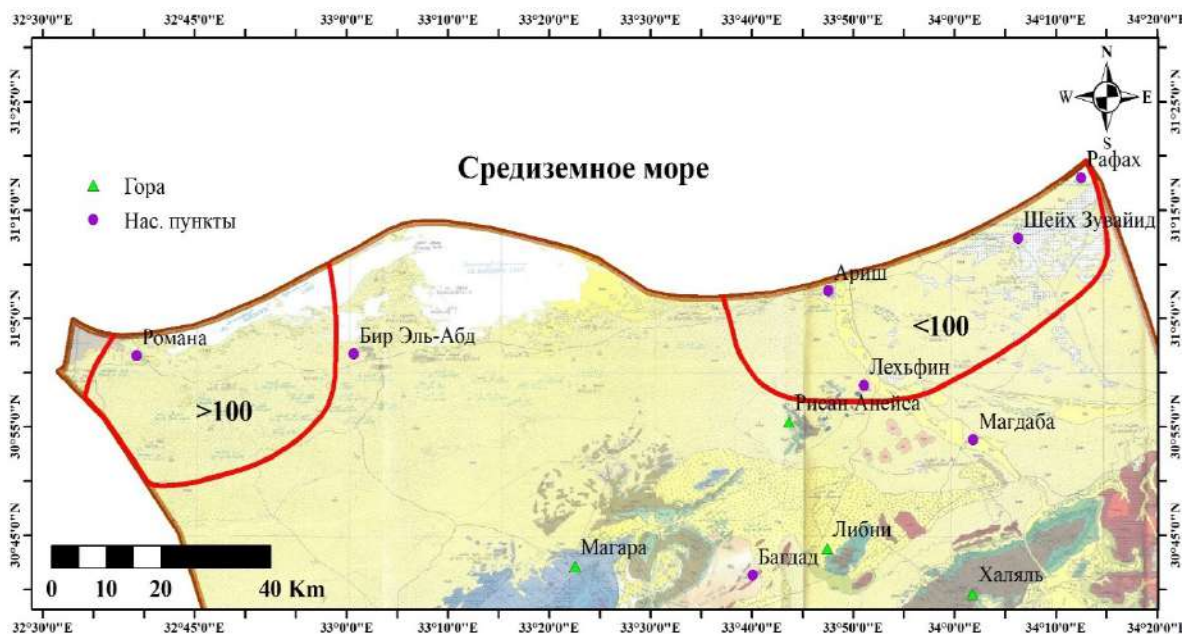
Fig. 3.22. Map of zoning the area of sand, according to the value of the filtration coefficient K , m/day
