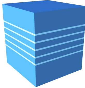
Figure 19: Structure of the sample ZMO1036 containing five ZnO/(ZnMg)O QWs.
