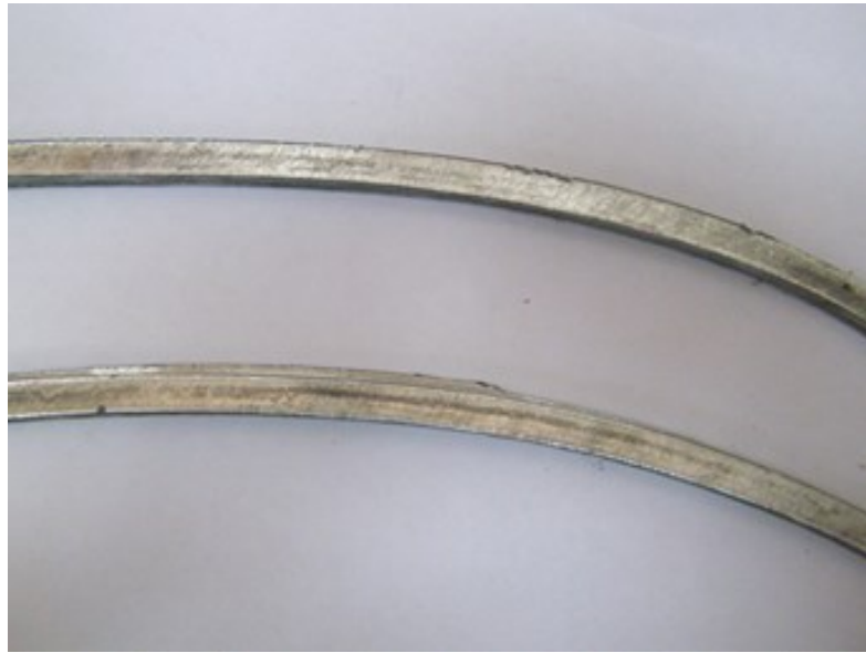
Figure 2.2.1. General view of blanks after processing of the 4th cycle by the ECAP-C method at 130°C along the route Bc.
