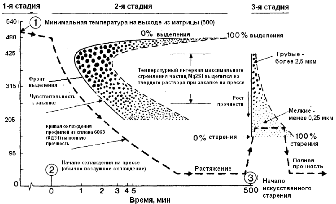
Figure 1.2. Scheme of separation of particles of alloy 6101 of different phases during aging ( t , min - T , °) [23].
