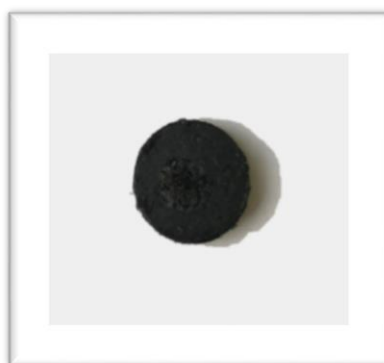
Figure 28. The pressed tablet based on silica and CNTs. Approach No. 3
