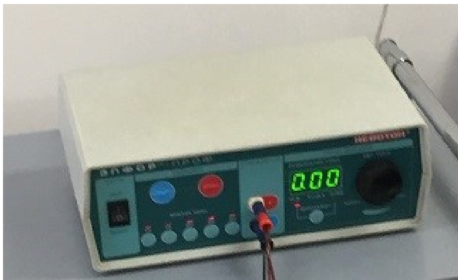
Figure 4 – Electroplating and medicinal electrophoresis device "PoTok"
