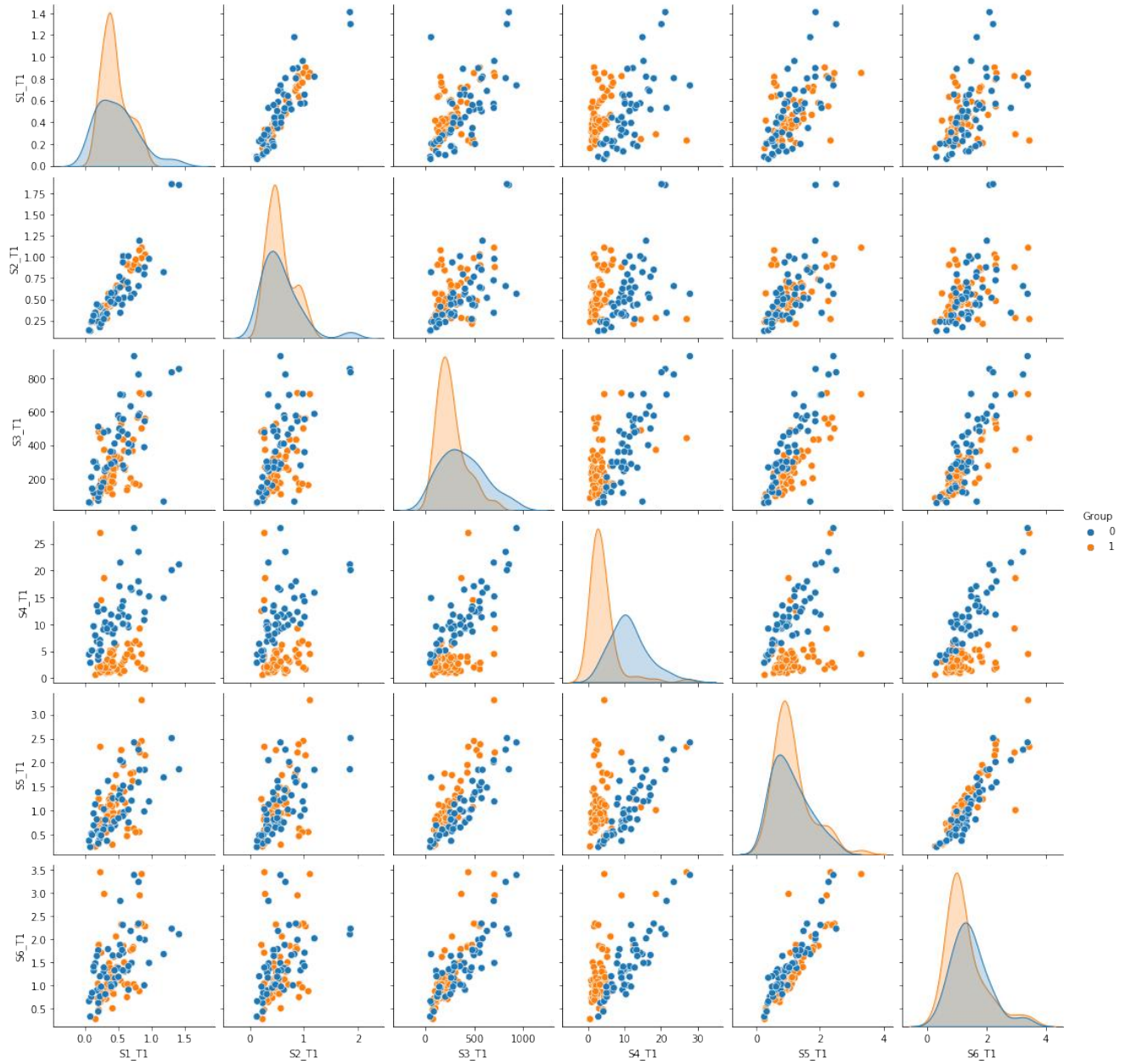
Figure 13. Matrix of scatter plots for 6 sensors at temperature mode T1. Cells (i,j) contain the scattering point diagram for the conductivity integral ( \mu\text{S}\times\text{s} ) of i and j sensors. The diagonal cells (i,i) show the smoothed distribution for sensor i. The grouping of the EB sample is shown in color (blue - control group (0), orange - LC group (1))
