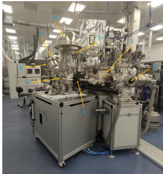
Figure 2.2. General view of the ESCA experimental setup: 1 - loading chamber, 2 - delivery chamber, 3 - analytical chamber, 4 - sample manipulator, 5 - X-ray tube with a monochromator, 6 - energy analyzer, 7 - detector, 8 - ion gun with argon inlet system.
