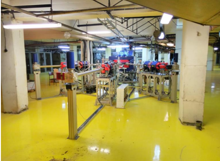
Fig 14. Wiring of beams to the target stations of the RIC-80 radioisotope complex, basement of the experimental hall of the C-1000 synchrocyclotron
