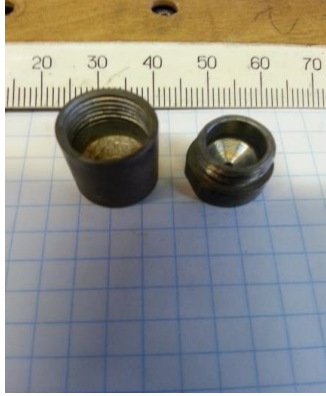
Fig. 24. Capsule after heating above 1123K (900 ° C). The target substance has completely disappeared.
